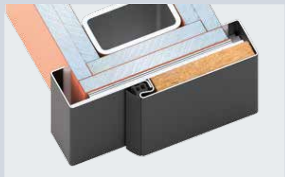
3. Screw counter frame profile of the frame to profile through the sealing groove and cover with the door sealing
